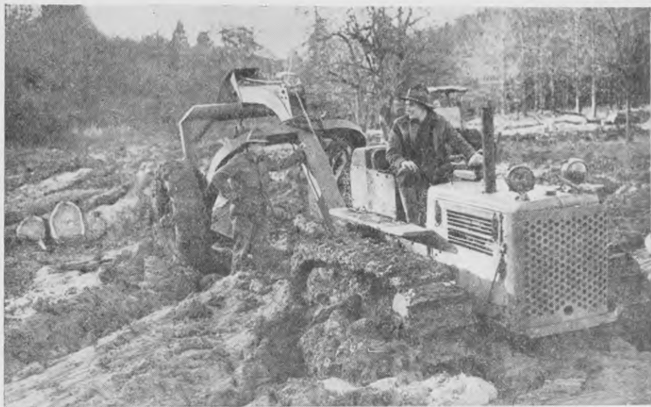
This Official War Photograph shows members of the New Zealand Forestry Corps in England using a tractor and logging arch to drag heavy timber away after felling.
