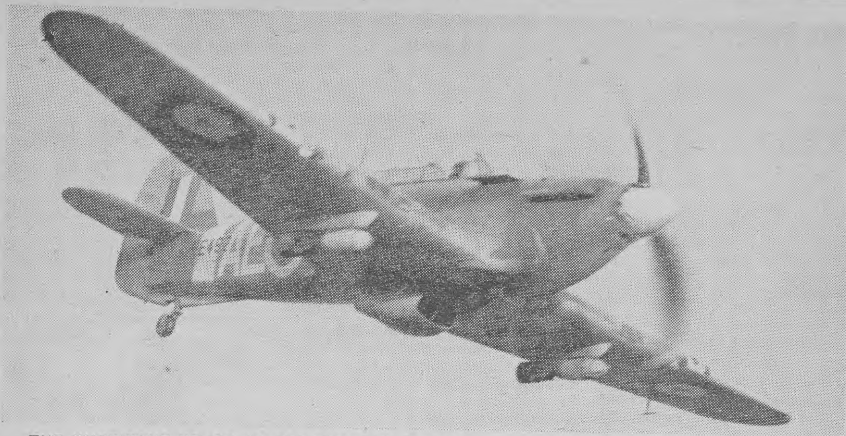
THE HURRICANE IIB, OR "HURRYBOMBER"—A Development of the machine which played a main part in the Battle of Britain, the IIB carries 250lb. bombs, and is armed with eight machine-guns. It played a major role in harrassing the retreating Axis convoys during the recent triumph in Tunis.
