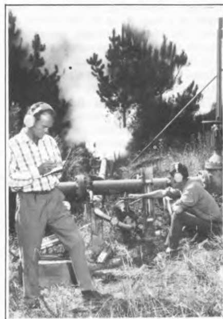
DSIR scientists check and record fluid flows at Wairakei in 1971. Flows are regularly monitored to check the performance of the field.
