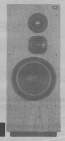
L100T: 3-way system with 300 mm low frequency transducer, 130 mm mid-frequency transducer, and 25 mm high frequency transducer. Sensitivity: 91 dB SPL, 2.83 V at 1 meter. Crossover frequencies: 800 Hz and 4.5 kHz. Maximum recommended amplifier power: 300 W. Impedance: 8 ohms. Dimensions (WxHxD): 406x925x322 mm. Shipping weight: 33.2 Kg each.
