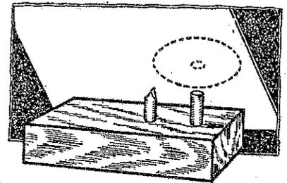
edges are just touching. When the circle has been completed the centre piece will fall out, and the circle can be trimmed up with a pocket knife.
