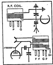
at the grid. Take your 2in. former and 3-16in. above the grid terminal drill a hole. The next hole is 3in. above the plate prong. Wind this space with 24 d.s.c. wire. Note particularly that the grid terminal connects with the bottom of the coil; it is unusual, but it is absolutely necessary in this circuit.
