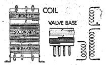
ally, in such a way that there is no mechanical connection. Thus we have a primary and secondary, and energy is transferred from the primary to the secondary without any connection between the two. It sounds rather wonderful, but it is one of the things that makes radio possible. To get the most out of a set, a coil, which possesses "inductance," and the condenser, which possesses "capacity," 'must be combined. When a coil of known induct-
