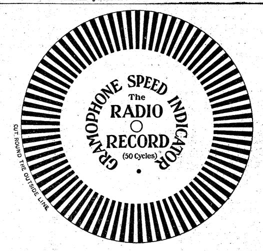
STROBOSCOPIC GRAMOPHONE SPEED INDICATOR. In response to requests we are reprinting this speed indicator from the 1930 Guide. Out out the disc and mount it on cardboard. Place it on the gramophone turntable and set the motor revolving. When viewed under electric light the bars should appear stationary. Adjust the speed regulator till this is so, when the speed regulator is the speed regulator till this is so, when the speed regulator till this is so, where the speed regulator till the sp
