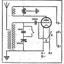
When using these on shortwave you must switch a series condenser of small value in the circuit, as shown in the diagram.
