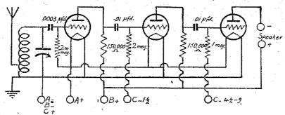
should rebuild the radio section of your set and use the improved method of transformer or tuned anode coupling
