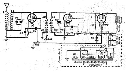
Theoretical Diagram.—The key to the parts not mentioned in the list are: R1, 425 ohms; R2, 200 ohms pot.; R3, 775 ohms; R4, 4700 ohms; R5, 25,000 ohms (not critical); R6, 100,000 ohms (not critical); R8, 50,000 ohms; R9, 500,000 ohms; R10, 20 ohms (not critical); C4, C5, 1mfd.
