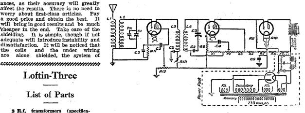
ier shields, with the remarkable results that the set became stable and workable. Aluminium not lighter than 18 gauge should be used, and foreseeing the difficulties in coil covers we have made arrangements whereby coils Their will be available from dealers. cost will be very small.
