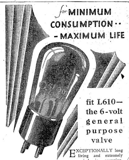
Specifications: Fil. volts 6.0 max. Fil. curr. 0.1 amp. Plate volts 150 max. Amp. Factor . 15 Impedance 7,500 ohms. Normal Slope 2.0 ma/volts
