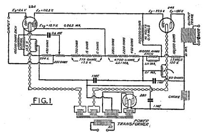
will considerably change the stability conditions of the R. F. amplifier. It is well known that the low dynamic input impedance of the grid leak detector assists materially in stabilising the R. F. amplifier, because of the damping effect which it has upon the tuned circuit connected to it. An R. F. amplifier which has been stabilsed for such a condition may no longer be stable when the detector is changed to a "C" bias detector without making proper changes in the R. F. amplifier.
