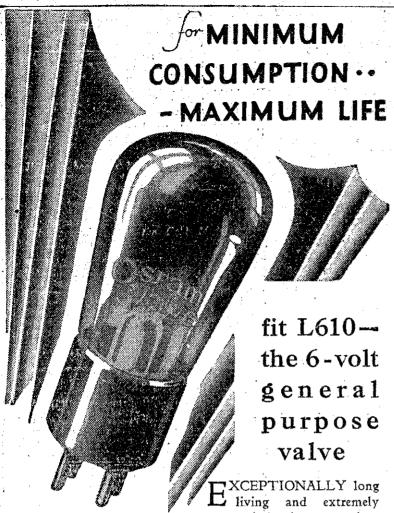
Specifications: Fil. volts 6.0 max. Fil. curr. 0.1 amp. Plate volts 150 max. Amp. Factor , 15 Impedance 7.500 ohms. Normal Slope 2.0 ma/volts Equiva-∫ A615 UX201
