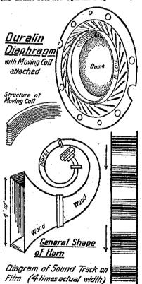
which ordinary thin wire is used. The coil consists of a thin aluminium ribbon 0.015in. (1/64) wide and 0.002 thick. This ribbon runs round a former which is afterwards removed, leaving the aluminium self-supporting with the turns adhering and yet separated by a film of insulating lacquer. The requisite number of turns is built up, and when complete is so compact that it resembles a ring made up of 22's brass sheet.
