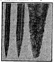
illustration shows the The top tapering point of the soft needle. can be readily understood why this needle will have less effect on the grooves of the record that the loud needle shown underneath. The lowest photograph depicts a rusty needle seen through a powerful mag-nifying glass. Its effect on the records is quite apparent.
