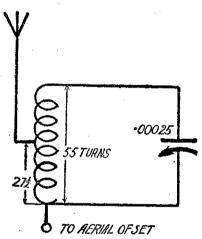
the station wanted, while reducing the strength of the unwanted station to the vanishing point. In building such a wave trap a little care must be taken, and although we will not go into the technical reasons here, suffice to say that the proportions given here should be strictly adhered to. Wind on a bakelite former 55 turns of No. for it is this that makes the success of this wave trap assured.
