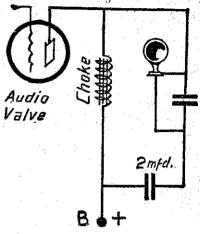
An output filter improves tone and saves the speaker windings.
