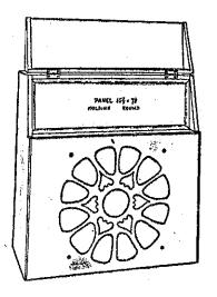
Inner frame ready for winding of frame aerial round outer surface. The small battens are to support the baseboard of the receiver, the space beneath this being occupied by the batteries and the back of the speaker.
