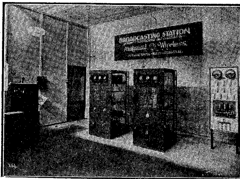
A.W.A. STATION 3EX, MELBOURNE. Showing Control Panel, Modulator, Oscillator, and Switchboard of this 500-watt Power Station.
