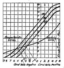
would oppose the negative electrons emitted from the filament, and reduce the current flowing in the plate circuit. while if a positive potential was an plied to the grid, electrons would be attracted to the grid and a current would flow in the grid to filament circuit. This is undesirable, as will be explained later.
