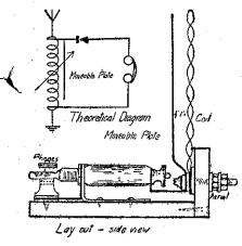
The tuning is affected by the distance that the copper disc stands away from the face of the coil, which should be from in. to lin. If the disc will not swing over the face of the coil, bend it away or remove a few turns from coil; if the loudest position is when the disc is full over, bend it loser until maximum volume is attained; move the disc with a piece of wood, not the hand, when tuning. The diagram shows the side view, with the theoretical diagram inset.
