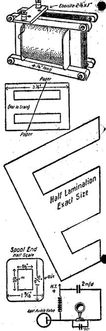
Then cut each square size, eighty pieces being right through on the diagonal line, The tin has the advantage afterwards cutting out the "window" pieces, bending the metal where necessary, afterward straightening out by Stalloy can be used, but edge of a flatiron, the point being held ening the cut plates is easy and effec-
