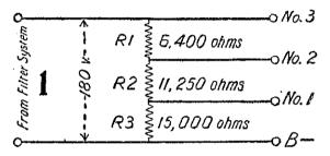
in order to make the total voltage between negative B and tap No. 2 equal to 90. The current flowing through the resistance R2, will be equal to the loss current of 3 milliamps, plus the current drawn by the detector, 1 mil-Therefore the value of R2 will be equal to the voltage (45) across it, divided by the current through it, which is 0.003 plus 0.001, or a total of 0.004 amperes. This gives a value of 11,250 ohms for R2.
