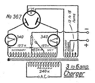
windings. For the primary winding. in place of 26's enamelled previously specified. In addition to previous recommendations it would be an adprimary winding, making the total 1065. As the filament winding has to must be used instead of 18's. The necesasry, but this would only be 1-8in. pose. or  $\frac{1}{3}$ in, at the most.
