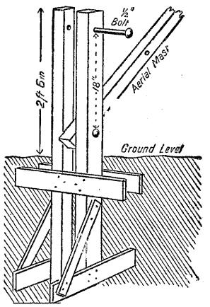
inches square being a suitable dimenuprights take a long half-inch bolt to B current to the plate of the valve. tion is kept within reasonable limits. act as a hinge. When the pole has been raised, it is held in place by a bolt passed through a hole drilled in each upright, and the pole, eighteen inches above the lower bolt.
