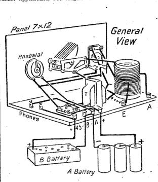
ply finished with shellac varnish rubbed in, makes a neat, inexpensive panel. On the front of the panel, which measures 12 by 7 inches, there will be the condenser dial in the centre, to the left the crystal unit
