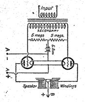
equivalent is provided by shunting the secondary with two high value resist-ances and making the grid-bias connection at the junction of the two.
