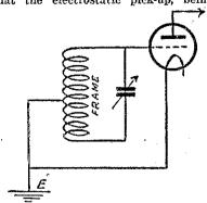
more or less evenly distributed over the frame, should be balanced out, leaving an approximation to pure electro-magnetic pick-up. The degree of success attained in eliminating the static pick-up can be gauged by the extent to which the local station can be eliminated by turning the frame into the position of minimum signals.
