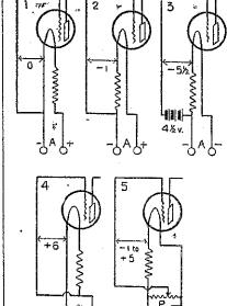
wire wound round a strip of mica. A 30-ohm, rheostat is connected in the positive filament lead. The above refers to operation from a six-volt battery, the voltage required for the filament being only 3.3 at .132 amps. For operation from a 4-volt battery, a 30-ohm rheostat is placed in the negative filament here the 10-ohm resistance is shown in the theoretical dia-
