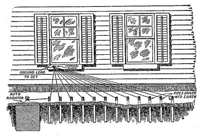
The account of Pierce's system said :- Outside the window there was something unusual. The wire that led from the ground connection on the receiver out through the window ended at a binding post on a porcelain base. From this post twelve wires led to the same number of pipes or other pieces of metal embedded in the ground (see illustration). Pierce said that he found that each new ground connection increased selectivity and reduced the effect of body capacity; so he added one after another.
