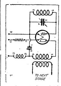
denser the operator has neglected to remove either a resistance or an inductance, which may have spanned the condenser, or the condenser is actually shorted. To make this clear, if the operator wants to test the variable condenser shown in the grid circuit of the tube in Figure 1, and places the test handles across the rotor and stator,
