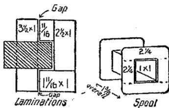
strip of strong millboard an inch wide is fastened by brads into the wood in the position shown by dots on the spool end. A hole in the centre of each takes the winding spindle.
