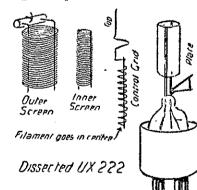
ducer, while the outer section (which has nothing to do with the stream electrons, because they stop at the plate), serves merely to reduce the capacity
