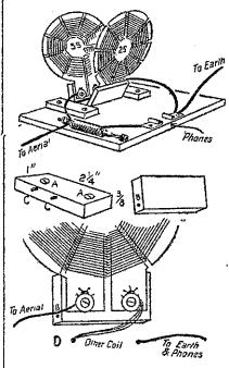
desired. If thicker wire than 20's is used, more turns will be required on the coils, as increasing the gauge de-creases the wavelength for a given
