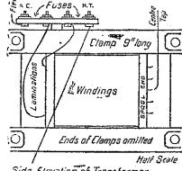
Side Elevation of Transformer
