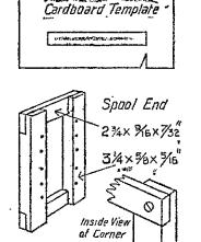
so that the joints do not come opposite. These should be assembled in a flat position. When most of them have been put in, and they begin to feel tight, the windings of the transformer can be tacked.
