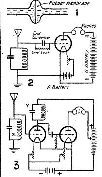
When the tube is required to act as a detector (that is, as a non-return valve) the characteristics required are
