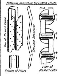
approximate only, and that they may be modified as found necessary. Unless the tubes are very full in size, the plates should be cut 11 inches in width to give minimum trouble in fitting. The separators can be put into the plain plates before the latter are put into the tubes, each pair down one side of the row to have a separator near the top of each, and those on the other side to have a separator near the bot-
