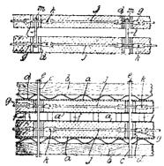
wall, sets of two tubes are placed in alignment, one in each part of the wall, each tube being of a length corresponding with the width of each of the parts of wall respectively. The plates or boards which form the moulds for the walls are tied together by rods which pass through the tubes which form distance-pieces between the outer and the inner plates or boards. After the concrete of which the walls are formed has set, the
