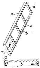
disposed transversely to each other, which ribs form a coffering. The slabs, plates, or the like are formed with depending ribs round their four edges, and with or without intermediate ribs, forming square or rectaugular inverted shallow boxer or depressions on the under side The depressions may take the form of double
