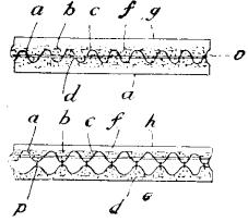
corrugated sheet so as to embed the wire netting and be securely held by the netting to the sheet. In some cases rods are passed transversely through the corrugations. The concrete may be stone, concrete, or coke-breeze. The work may be finished off with neat cement, rough-east, plaster, or otherwise,
