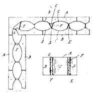
members. These wire ties are embedded in the block during the moulding thereof.
