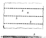
ity of layers of thin board or veneer united together by means of stitching of thread, twine or the like. Grooves may be formed in which the stitches are laid,
