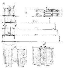
consists of special cramps, either in one or several pieces, for adjusting to various thicknesss of wall or walls. Bands in one piece or in more for the purpose of adjusting to the sizes of walls or studs, for supporting studs that in their turn support the boxes or formes, are also employed.
