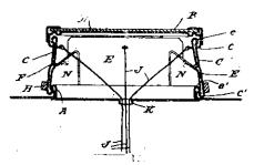
extending along each of its sides, and in providing a cover for such opening that is pivotally supported in the frame so that it may be turned to uncover the opening or may be left free to cover it.
