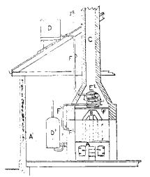
baffling-hood over them. These are placed immediately above the range or fire flues in a convenient part of the usual chimney and water so heated is led down to the usual hot-water cylinder, or otherwise as preferred.
