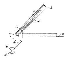
attached that serve to counterbalance the weight of the frame. This weighted counter-balance will thus allow of the skylight being opened by any of the ordinary appliances, with great facility, and will also serve to maintain it at any position to which it may be raised.
