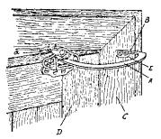
of the friction-grip type for retaining hinged doors in open or partly open position or in closed position as may be re-
