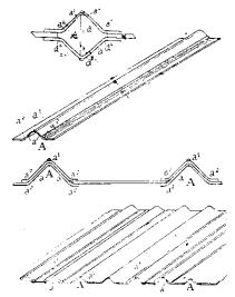
whilst maintaining the thickness of the material constant. This form comprises a large corrugation with straight sides at an angle of preferably about 45° to the horizontal and 90° to one another, and the apex and base curved or rounded off to permit one to bed or lie flat upon another (or any modification thereof between 30° to 60° to the horizontal and 60° to 120° to one another), and with each corrugation
