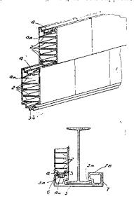
on one edge of the block a tongue, and on the other edge a groove of approximately corresponding design, the groove being substantially larger than the tongue to provide extra room for cement.
