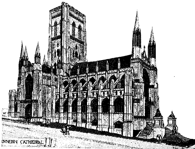
Revised Perspective Drawing of Dunedin Cathedral, showing fine entrance steps, with statuary, flying buttresses and other features not shown in the original perspective.
