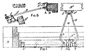
slide in and out on a rod A on the sash frame upon the operation of pull cords E2. An automatic catch D2, which is released by the pull cords, holds the fan-light in the closed position.
