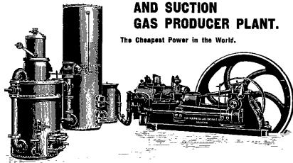
A 25-b.h p. at Wanganui works on 111bs of coke per horse-power per hour. A 40-b.h.p, installed for Messrs. Lind & O'Connor, Flaxmillers, Shannon, is now at work. All interested are invited to inspect.
